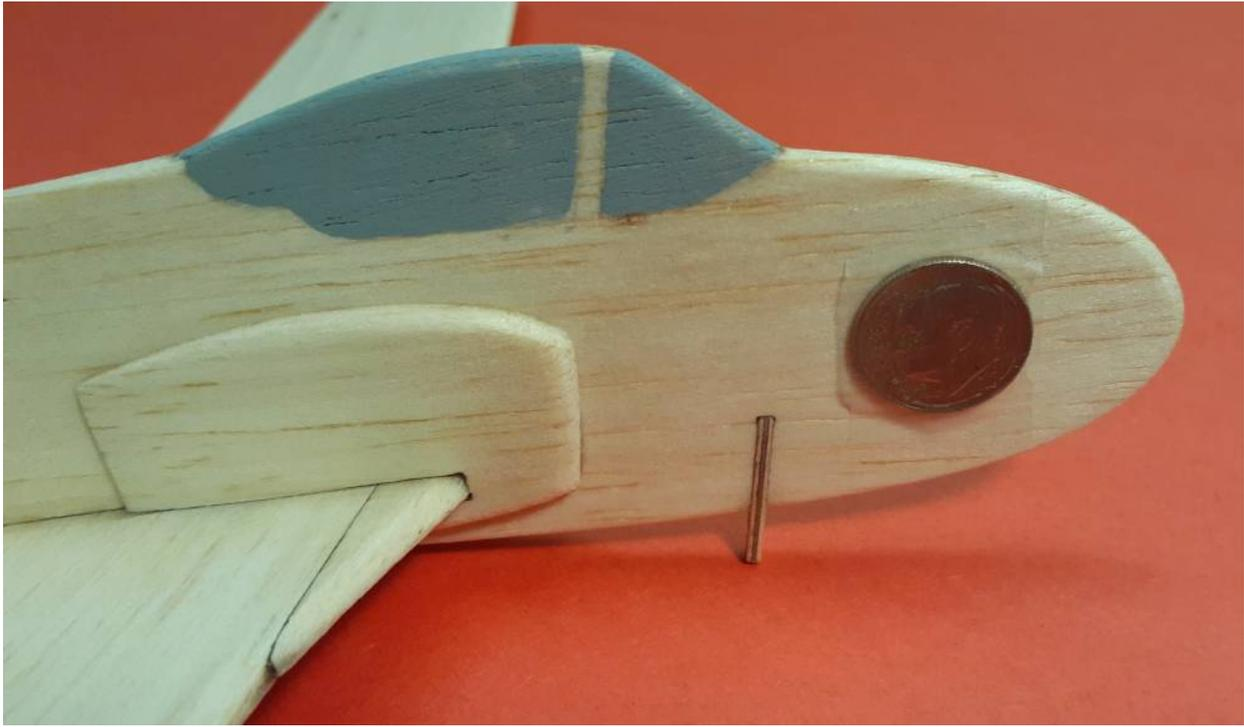
Throw the glider with the wings level and the nose slightly down. Try to throw it just fast enough for it to glide away from you steadily. If the model dives downwards, move the dime a little further back. If the model climbs and then dives (stalling), move the coin further forward. If needed, add more weight using modelling clay. Aim for a slow glide with a nice smooth flight.
