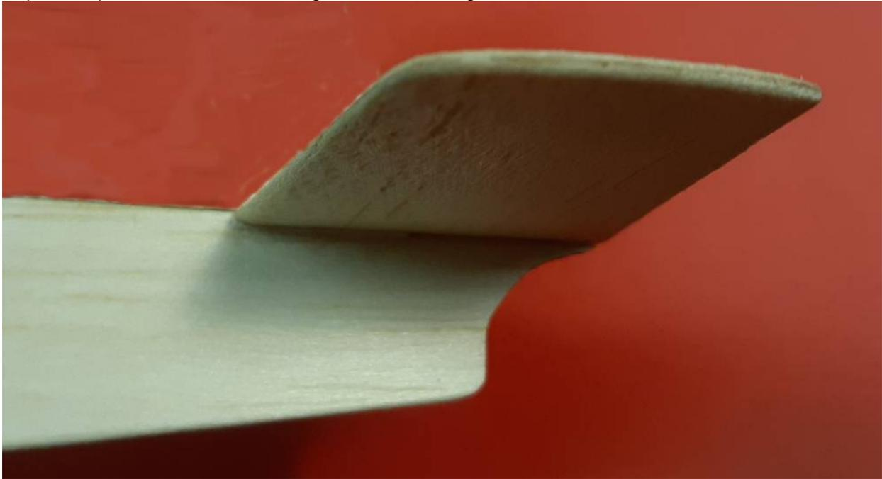
Check that the tail fin will fit closely on top of the fuselage and tailplane. Sand if required. Then glue the tail fin to the top of the fuselage and tailplane. Make sure that it is vertical and exactly in line with the fuselage and tailplane center line.
