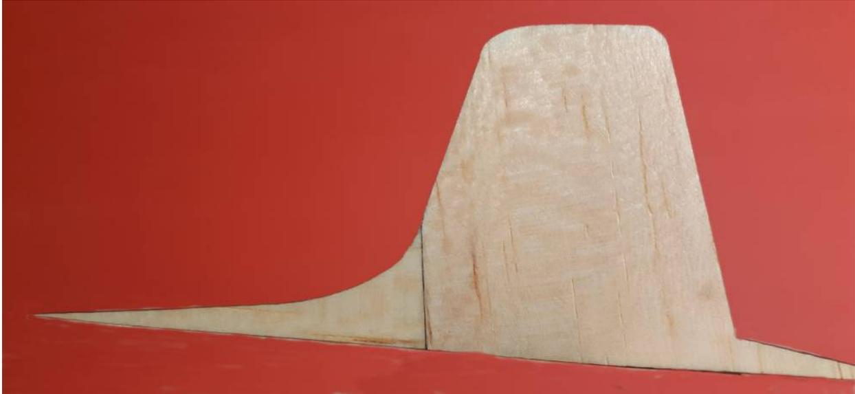
Slide the tailplane onto the rear of the fuselage. The slot goes toward the front so that the tailplane goes all the way forward. The top edge of the tailplane will align with the top edge of the fuselage. Glue the tailplane in place so that it is at 90 degrees to the fuselage side.
