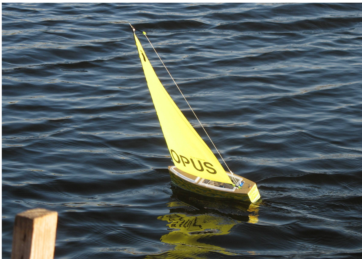
Here the rig is set for a little more wind, so a little more manual twist.
