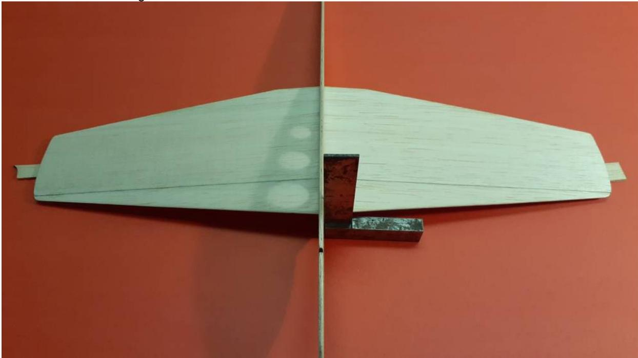
To check this, you can set the fuselage and wing inverted on a flat surface. Use a right angle to set the fuselage vertical. Put a scrap of 1/8" (3mm) balsa under each wing tip. When satisfied with the alignment, run thin superglue along each side of the joint to glue the wing in place. Glue on the top surface when the glue is set.
