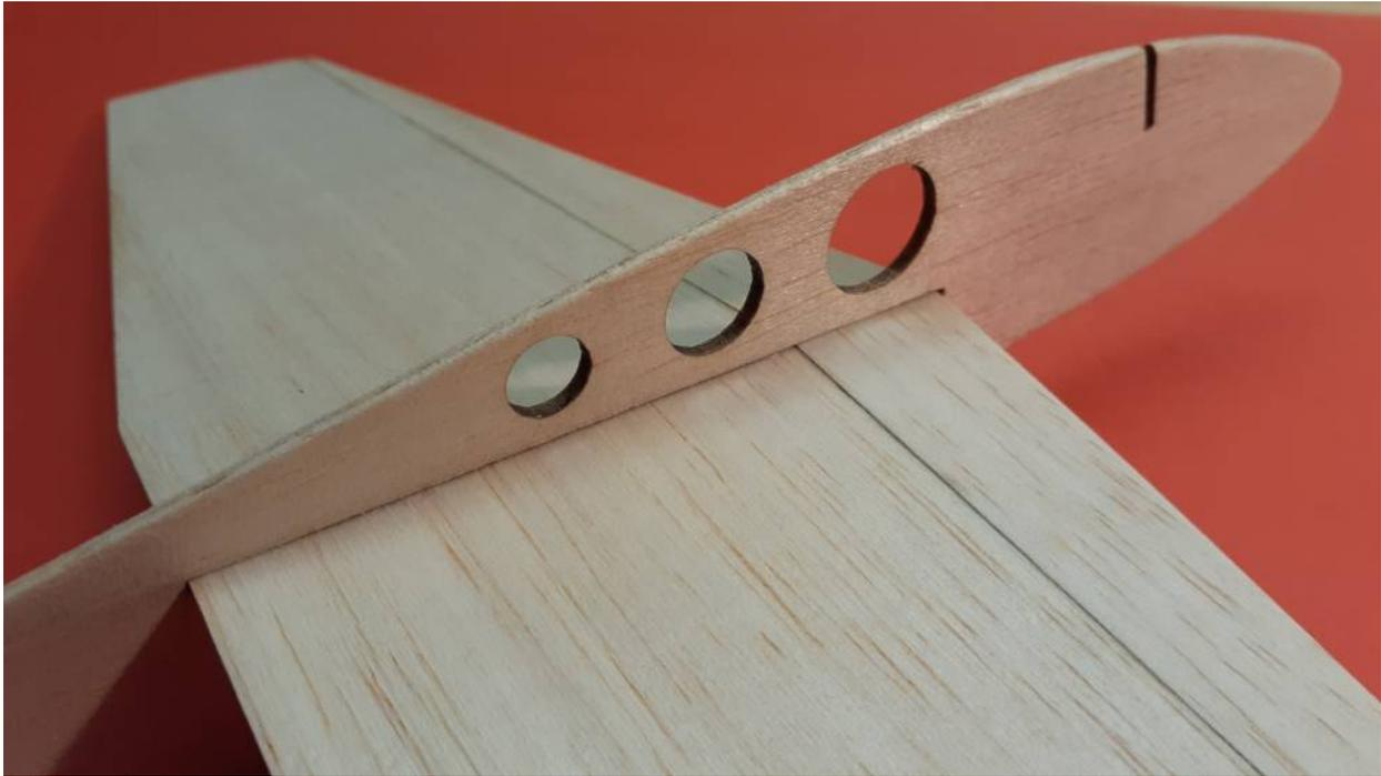
Look from the front of the fuselage; the wings should be positioned so that they are at the same angle on each side of the fuselage.
