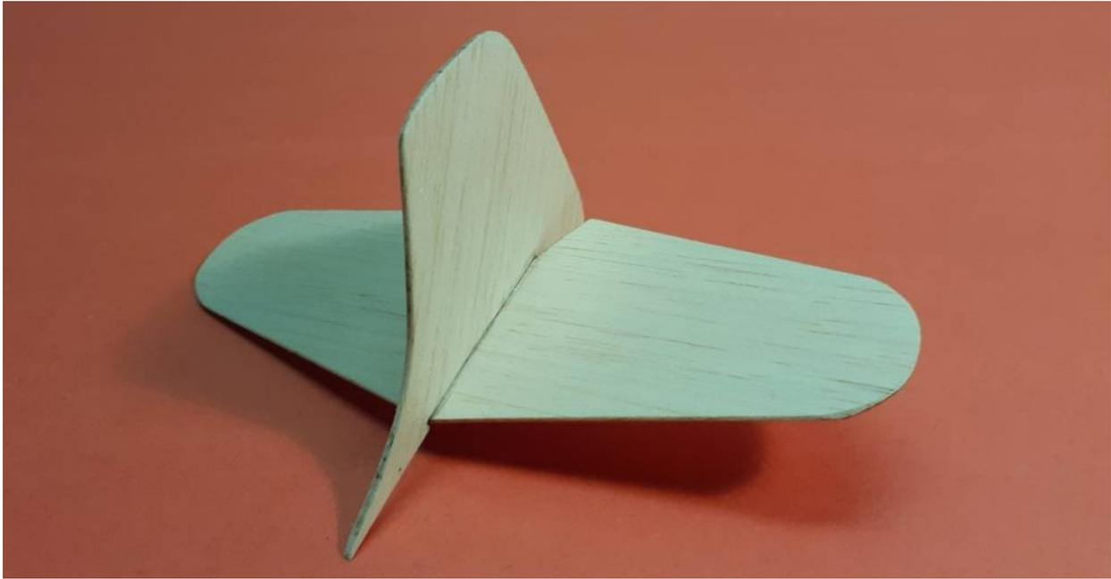
Position the tailplane and fin on the rear of the fuselage. The top edge of the tailplane will align with the top edge of the fuselage and the rear of the fin will fit to the rear edge of the fuselage.
