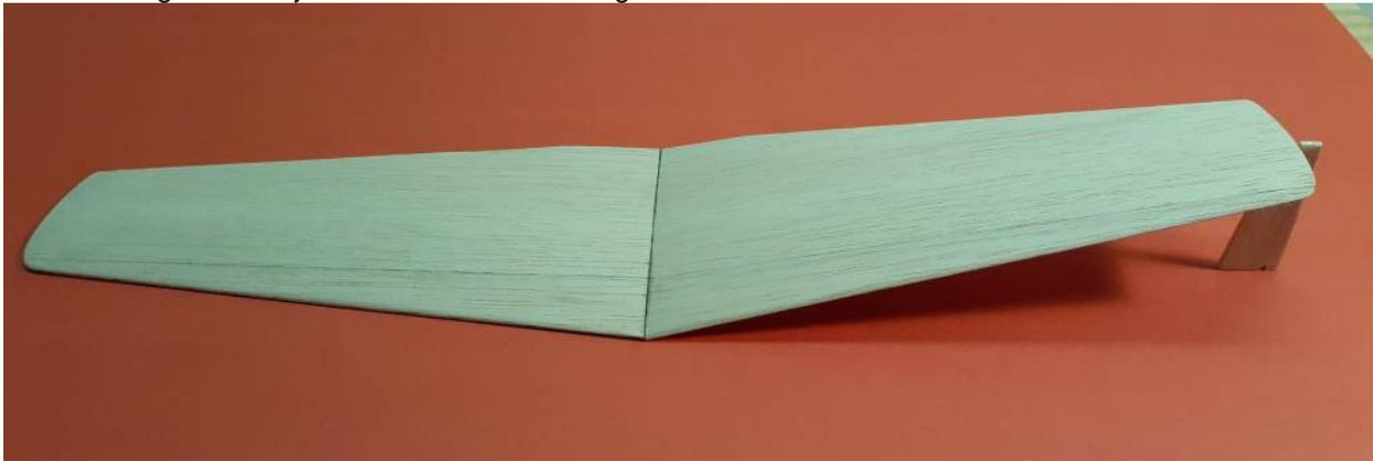
Next put one wing flat on your board. Prop the other wing tip up  $1\frac{3}{4}$ " (45mm). Once you are satisfied with the alignment, apply glue and leave to dry. A handy tip is to stick a strip of packaging tape to your board and make the glue joint over that.
