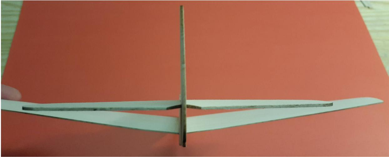
Glue the plywood catapult peg into the slot in the fuselage.
