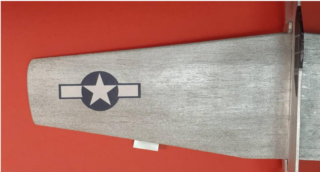
The aircraft markings are applied in the same manner. The larger insignia goes on the left wing, both top and bottom. The smaller insignia go on each side of the rear fuselage. Lightly brush a thin coat of Shellac over the paper decals to protect them.
