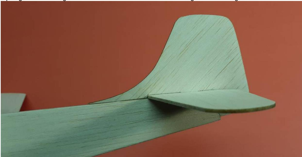
When you are satisfied with the fit, glue the assembly onto the fuselage. Make sure that the fin is vertical and exactly in line with the fuselage center line.
