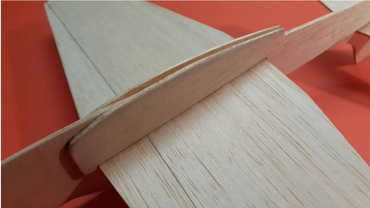
Slot the tail fin into the tailplane. The tab will help with the alignment.
