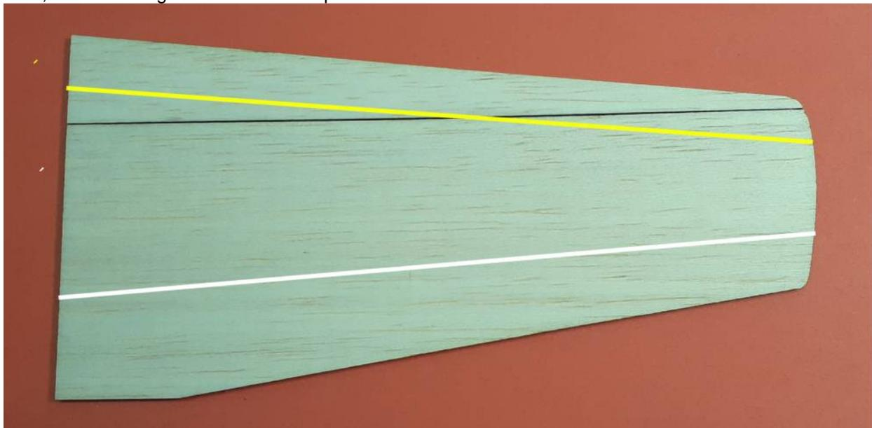
Take your sanding stick and sand the top front edge of the wing in a curve down to the bottom edge. Start this about 1/2" (12mm) back from the front edge (yellow line). Then round the bottom corner of the front edge. Do this along the whole length of one wing panel.
