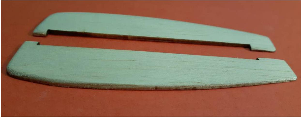
Take the two engine nacelles and sand toward the rear edges so that they taper to about 1/16" (1.5mm) thick. Be sure to make both a left hand and a right hand nacelle. Round off all of the outside edges.
