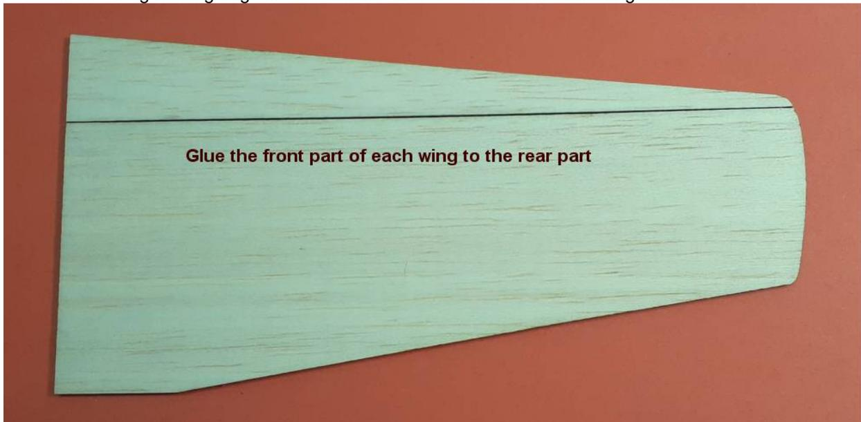
Next, sand the wings to an aerofoil shape.
