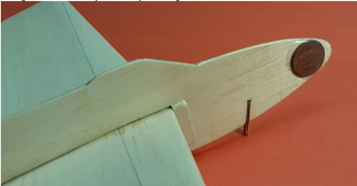
Throw the glider with the wings level and the nose slightly down. Try to throw it just fast enough for it to glide away from you steadily. If the model dives downwards, move the dime a little further back. If the model climbs and then dives (stalling), move the coin further forward. If needed, add more weight using modelling clay. Aim for a slow glide with a nice smooth flight.
