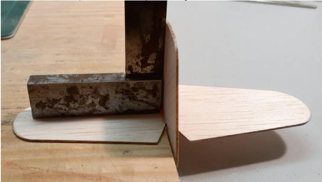
Set the fin at the edge of a board and use a right angle to get the fin at 90 degrees to the tailplane. Glue in place with superglue.
